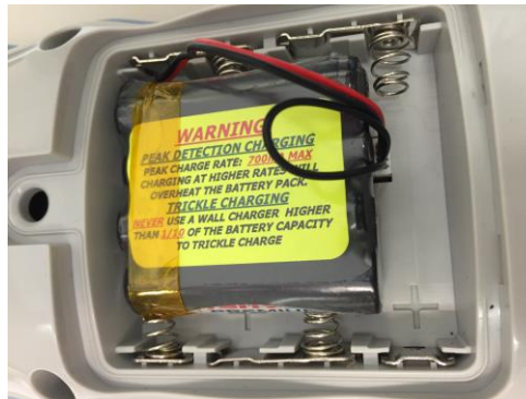
Figure 3-2: Installing Rechargeable Battery
