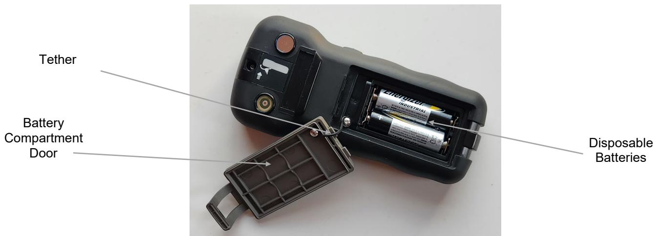
Figure 3-1: Installing Disposable Batteries
